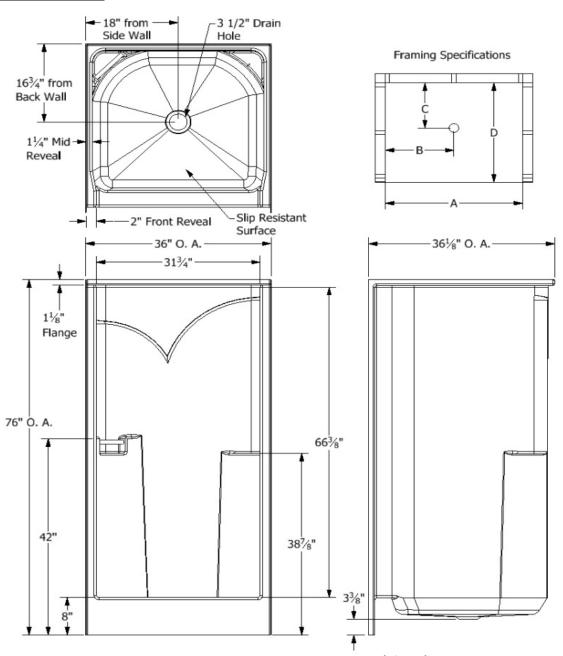
Certified to conform to HUD/UM73b,ANSI Z124.1, and ASTM E- 162 Flame Spread Rating 200 or less and is under a program of factory inspection.
